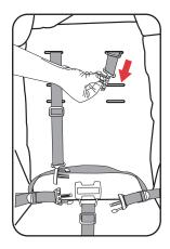
H To reposition the harness, pull the shoulder harness buckle tongue through the desired slot.
