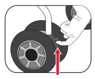
B Push the locking clip down to allow the wheels to swivel.
