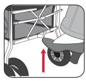
C Then depress and release the secondary lock with your foot and push handles forward until the frame is fully folded.
