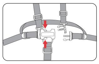
F To release the buckle. Squeeze the top and buckle tongues together with enough pressure so the buckle tongues can release from the buckle housing.
