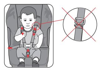
E Tighten or loosen the shoulder straps, slide the 3 bar slider up or down to adjust to the desired fit. Always adjust the harness strap when changing the seating position of the child.
