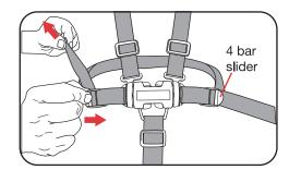
D Tighten or loosen the waist straps, hold and lift the 4 bar slider and then pull the harness strap, to adjust to the desired fit. The waist strap needs to fit firmly around the child.
